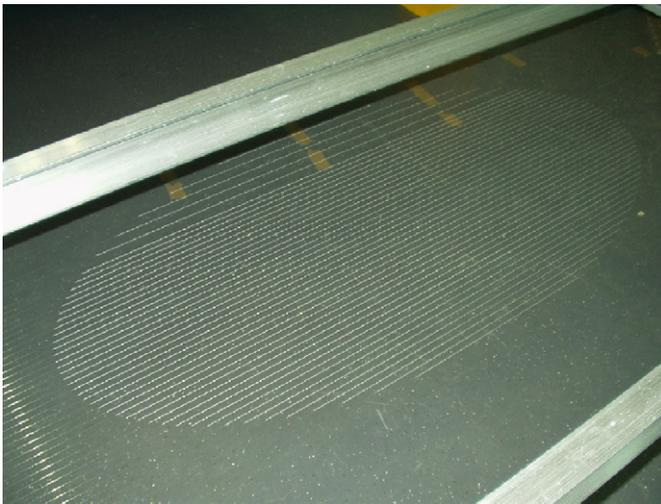
Fig. 32. The dead region of a large area drift chamber. In the central part of the chamber (diameter 1 m) the sensitive wire thickness is five times larger than in the active part of the chamber.
